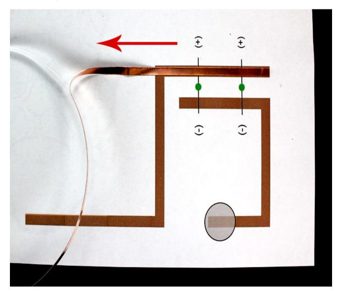
Apply the copper tape in a straight line and then bend it up at a 45 degree angle.
