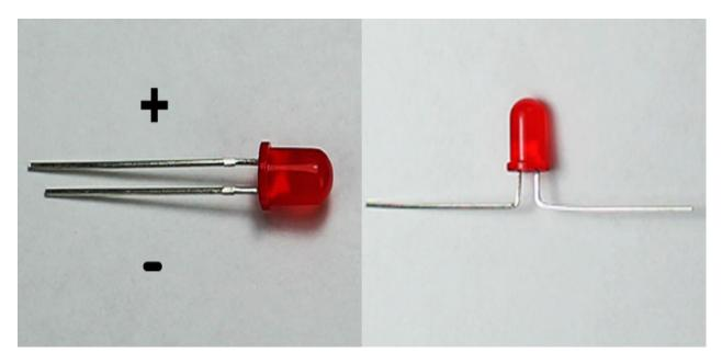
Mount the LEDs to the template making sure the long leg goes on the (+) side. Use copper tape to secure the legs to the copper tape below. Rub the copper to make sure it is making a solid connection.
