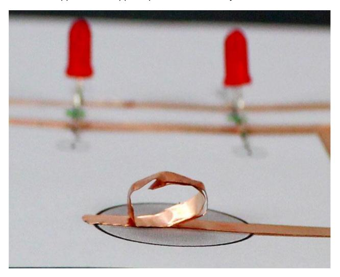
Place a CR2032 battery on top of the copper roll with the negative (-) side facing down.
